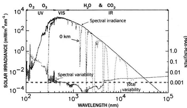
Fig. 3. Observed spectral solar irradiance at the top of the atmosphere and its estimated variability along the 11-year solar cycle. Also shown are the irradiance spectrum at the Earth’s surface (0 km) and the main gases absorbing solar radiation (taken from Lean, 2000). The horizontal dashed line corresponds to the TSI variability observed along the solar cycle.
